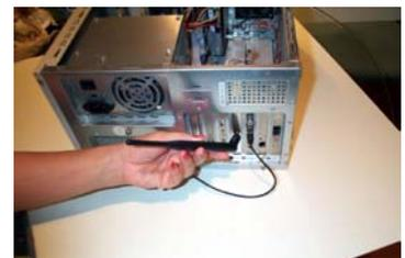
Twist on the antenna at the back of the WL-660 PCI card carefully
