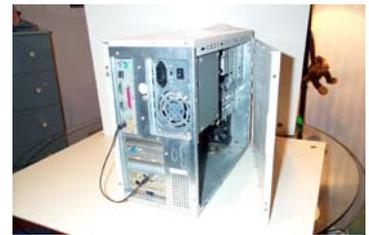
Pull out the side panel gently and find an empty PCI slot at the motherboard
