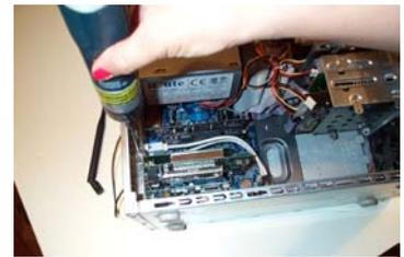
Insert the WL-660 PCI card and fasten it with the screw
