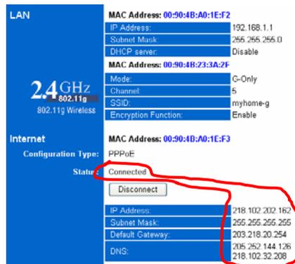
The "Status" screen refreshes every six seconds. It shows a bunch of IP and DNS addresses if the AP router is connected to your ISP
