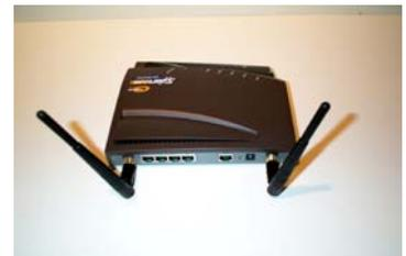
Twist the dual detachable antennae on to the AP Router. Each antenna has a 2dBi RF signal sensitivity gain
